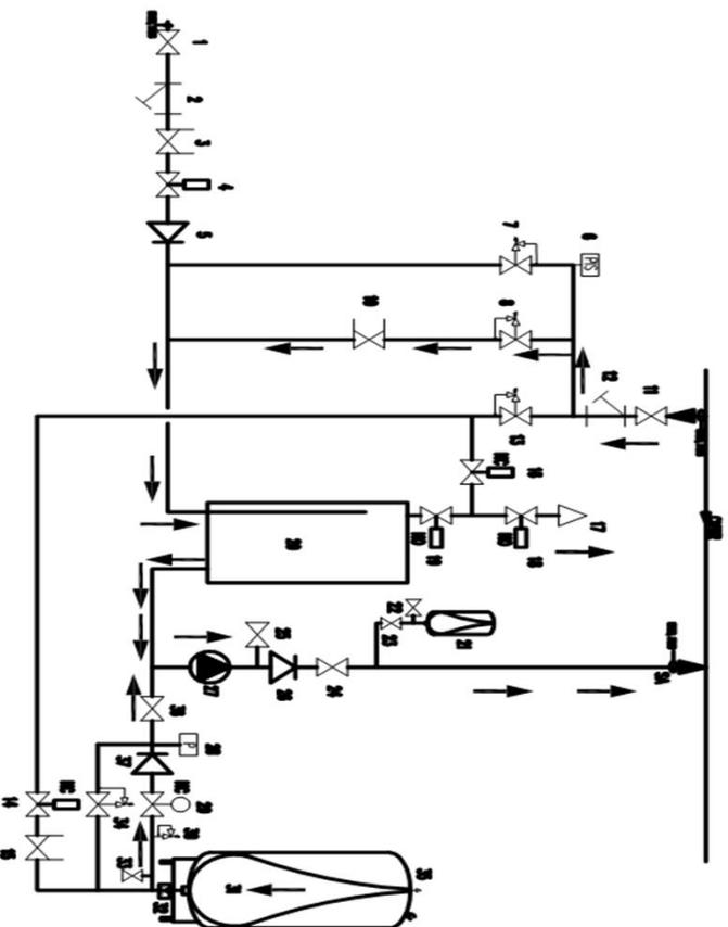
System pressure is lower than target pressure: pump(s) (27) is on, pressure reducing valve (8) opens, control valve (29) open slowly, control valves (16) (18) (19) close/open regularly to move air out to the system. Water from from system to air separator at vacuum pressure, air is removed from water and go to valve (19) (18) (17) to go out. Another flow from main tank (31) to (30) (29) (37) (36) (27)(26) (24) to go to the system to keep pressure of system stably
