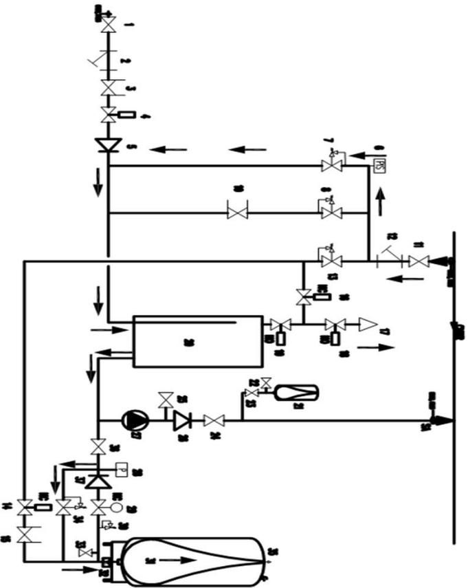
System pressure is higher than target pressure: pressure relief valve (7) (34) open, water from chilled water system goes to main tank (31)
