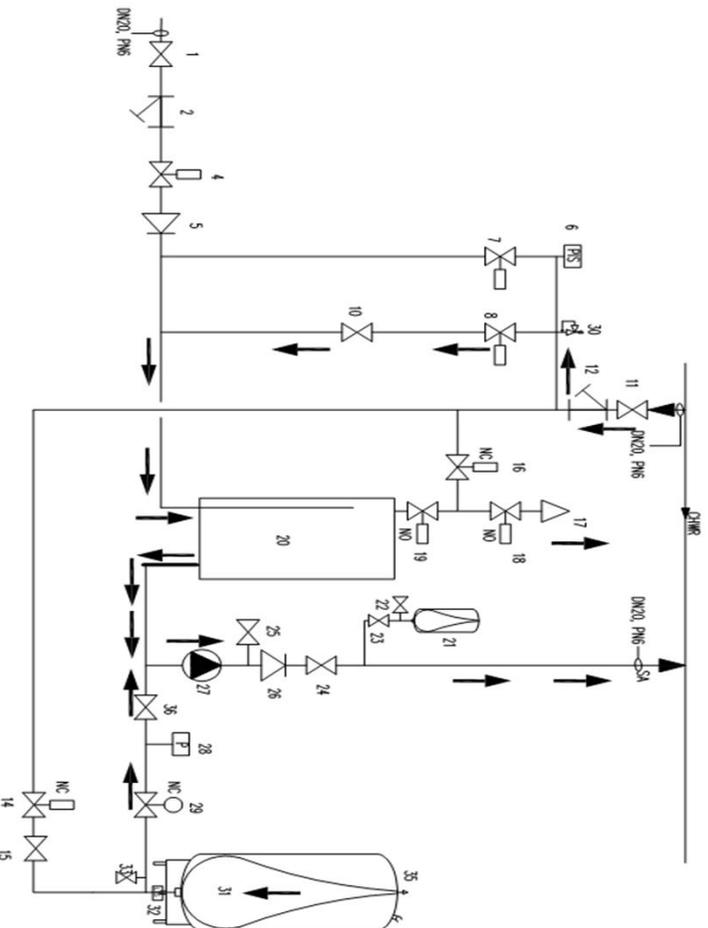
System pressure is lower than target pressure: pump (27) is on, motorised on/off control valve (8) opens, motorised modulating control valve (29) opens slowly, control valves (16) (18) (19) close/open regularly to move air out to the system. Water from from system to air separator at vacuum pressure, air is removed from water and goes to valves (19) (18) (17) to go out. Another flow from main tank (31) to (29) (36) (27) (26) (24) to go to the system to keep pressure of system stably
