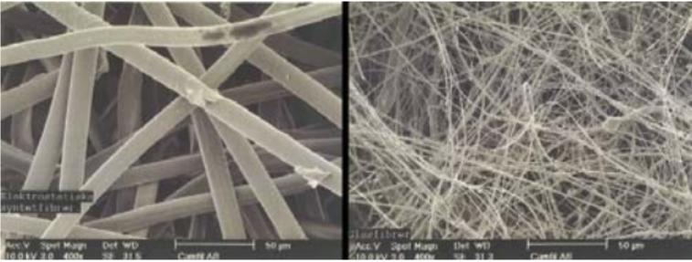
The magnified image on the left is MERV 13 synthetic coarse fiber media. The image on the right is MERV 13 fine glass fiber media. Economical to produce, coarse fiber media is dependent upon an electrostatic charge to obtain a MERV 13 rating. The charge disappears as the fiber loads with dirt. The fine fiber media uses mechanical principles of particle capture ensuring that the filter will maintain its efficiency over time.
