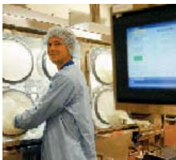
The glovebox is maintained under negative pressure.
