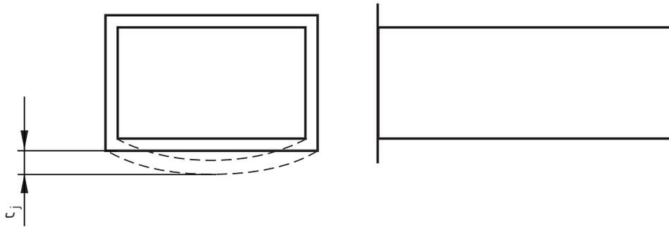
Figure 3 — Deflection of a joint
