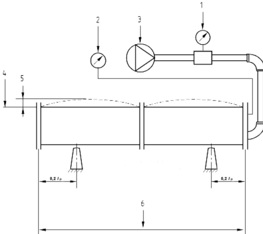
The accuracy of the measurement of support distances shall be within  $\pm 5$  mm.
