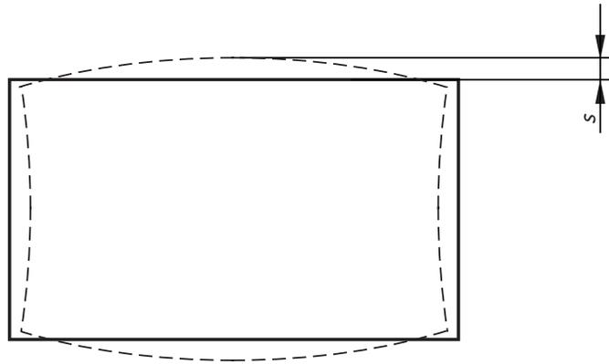
Figure 4 — Bulging/caving
