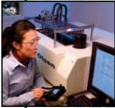
We manufacture two models that perform Deflection Temperature Under Load (DTUL, also called Heat Distortion) and Vicat penetration tests, with six and three test stations respectively. The larger machine can test up to six different specimens simultaneously, with an automated test sequence that proceeds according to user programmed control and configuration parameters.
