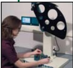
Our IT503 and IT504 Impact Testers feature heavy-duty construction with an aerodynamic compound pendulum, ensuring maximum rigidity in the direction of impact. This unique construction virtually eliminates windage losses yet allows simple and rapid changes in capacity by adding or removing weights on the pendulum. The proper accessories allow these machines to operate in accordance with ASTM D 256, D 6110, D 4812, D 4508, D 950,
