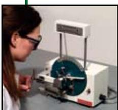
Tinus Olsen Stiffness Testers are ideal for determining the stiffness properties of a wide range of materials and products. Operation is simple; a specimen is clamped at one end and a controlled load applied at the free end. The load is applied steadily by a motor drive, and an accurate indication of load and resulting angle of bend are shown simultaneously on analogue scales.
