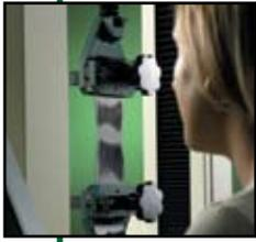
Tinius Olsen's versatile benchtop polymer testing machines can perform many materials test routines that meet ASTM, ISO and other international specifications, including tensile, compressive, tear, peel, flexural, puncture, shear and frictional resistance tests. Several different machines are available at five load tier points, namely, 1 kN (225 lbf), 5 kN (1,125 lbf), 10 kN (2,250 lbf), 25 kN (5,625 lbf), and 50 kN (11,250 lbf).
