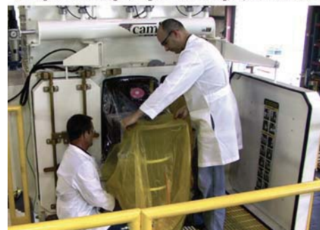
Surrogate tested bag-in/bag-out safe change option available.
