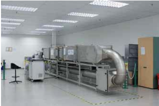
The Camfil Malaysia facility provides testing data for our customers and is used for research to support progression in the development of filter testing standards.
