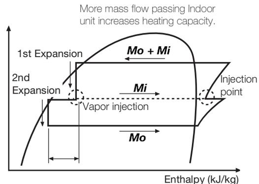
Vapor injection reduces the liquid enthalpy in flash tank, facilitating heat exchanger to absorb heat more.
