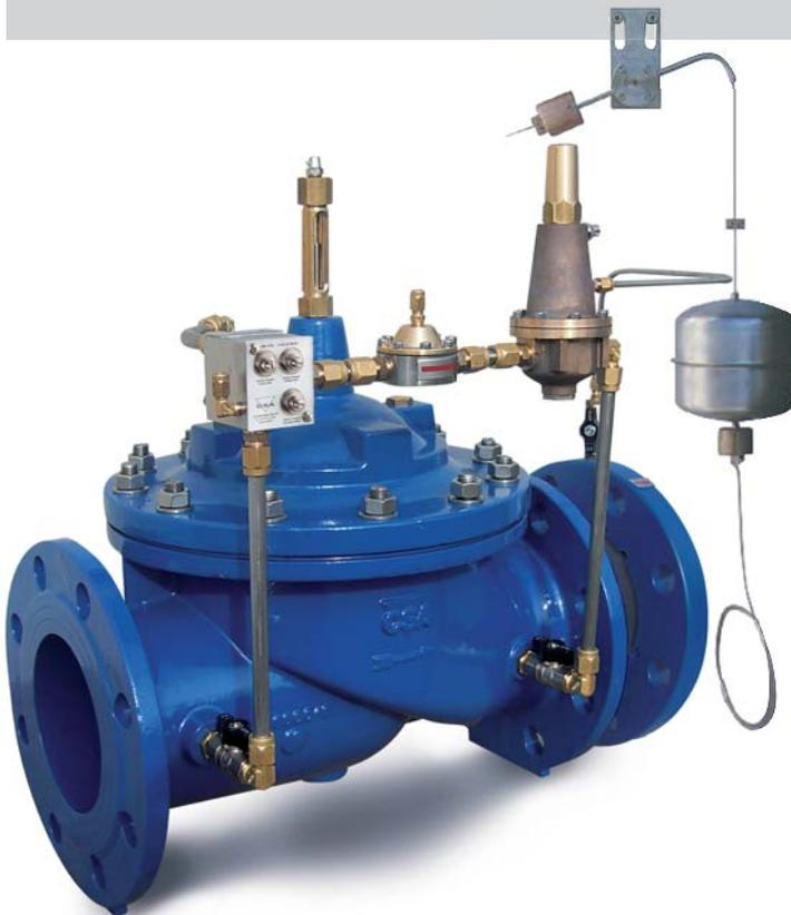
The CSA XLC 434 level regulation flow control valve limits the flow to a requested set point, regardless of pressure variations. At the same time, thanks to a three ways on-off level control pilot CSA mod. Rotoway, she controls the minimum-maximum level inside a tank. During the opening phase of the pilot, in case of flow rate lower than the set point the valve will be fully opened. For the proper installation the flanged orifice, supplied with the valve, must be placed at least 5 DN downstream.
