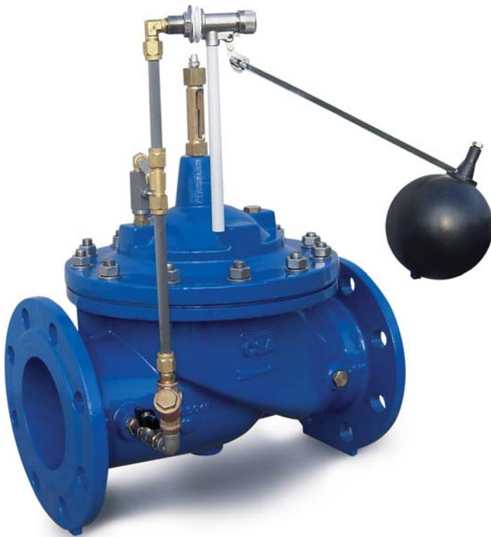
The CSA XLC 460 constant level control valve will automatically maintain the tank level within a range of approximately 15 cm. Thanks to a CSA needle valve the reaction time can be adjusted, to prevent water hammer effects during the closing phase. It is important to follow the instructions enclosed in the set up and installation manual, for the proper layout and minimum pressure required.
