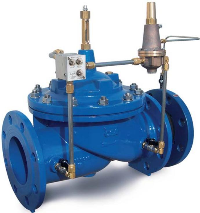
The CSA XLC 430 flow control valve will automatically limit the flow to a preset value, regardless of pressure variations. In case of flow rate lower than the required set point the valve will be fully opened. For the proper installation the flanged orifice, supplied with the valve, must be installed at least 5 DN downstream.
