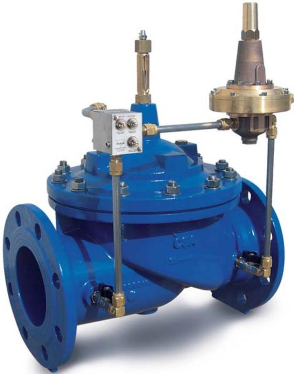
The CSA XLC 470 altitude control valve will maintain the level of a water tower or a tank, regardless of upstream pressure variations, acting with an accuracy of few cm of water column.
