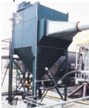
Pulse Discharge of Gold Cone Filter
