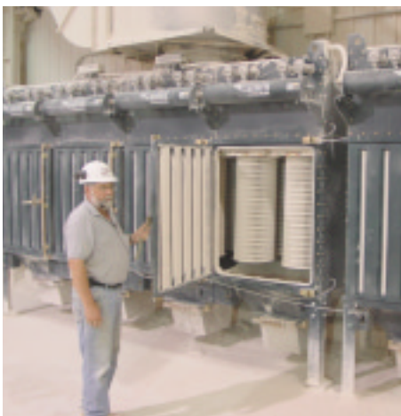
Louvered door inlet for cross-flow applications
