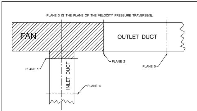
If the fan and system check out, begin testing the fan. There are five critical measurement groups that must be made to get the most accurate air performance test:
