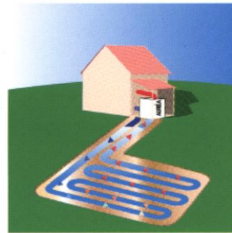
A horizontal underground loop system.
