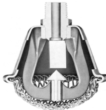
FIGURE A.3.3.6.4 Foam-Water Spray Nozzle.
