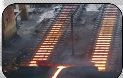
铸铁机 Pig machine
