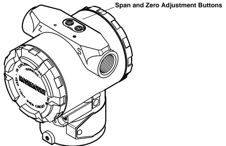
After you rerange the transmitter using the span and zero adjustments, it is possible to disable the adjustments to prevent further reranging. Refer to “Local Span and Zero Control (Local Keys)” below for more information.
