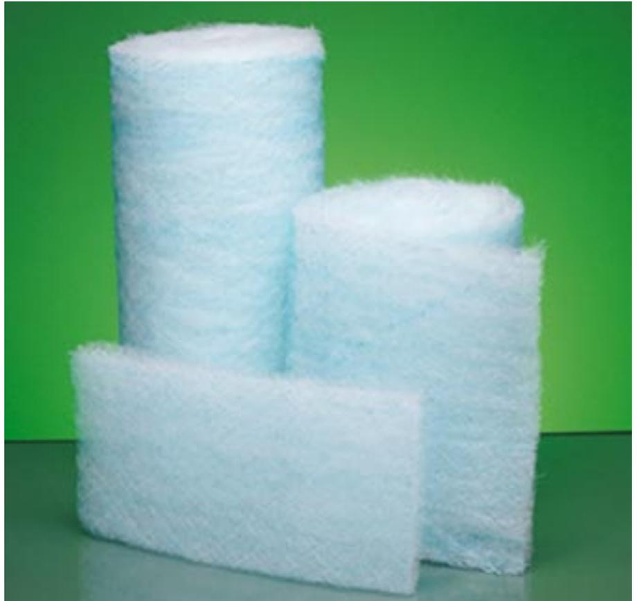
AmerGlas PaintStop Green is a commercial grade media designed to remove paint overspray in paintspray cabins. The filter media is made of continuous filament glass fibres with an open weave pattern that allows particles to penetrate deep into the pad. Paint is collected throughout the full depth, extending pad life and reducing costs. This exclusive media design eliminates faceloading, increases arrestance and ensures cleaner air.
