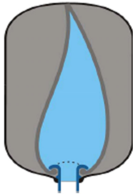
Figure 3.61 Expansion tank with a bag. Courtesy of TA Hydronics
