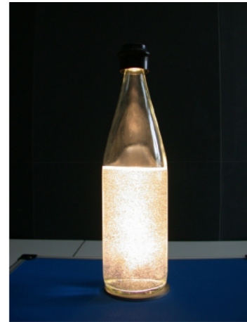
Figure 3.72 Microbubble separation by pressure reduction. Courtesy of TA Hydronics
