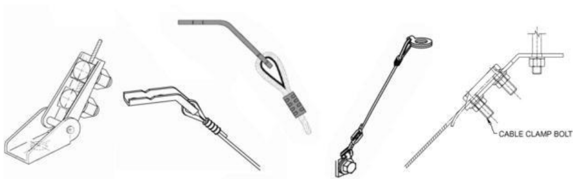
Figure 5. Types of Cable Connections
