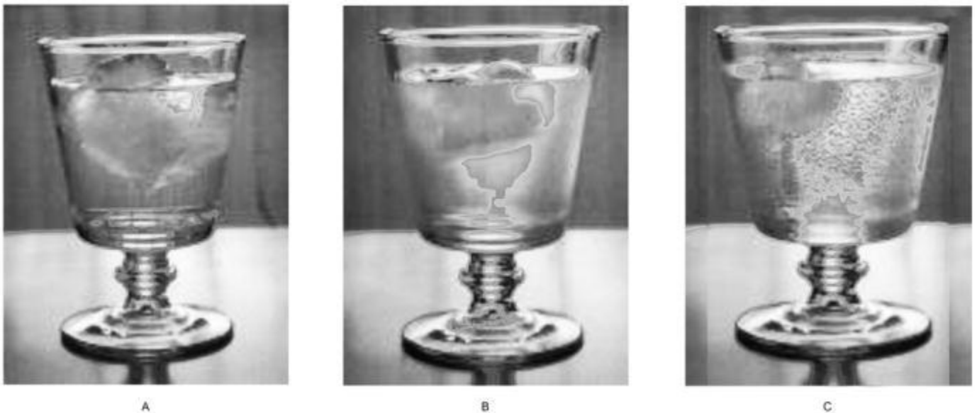
Figure 2. Stages of Moisture Condensation on Glass (Courtesy Desert-Aire Corp)
