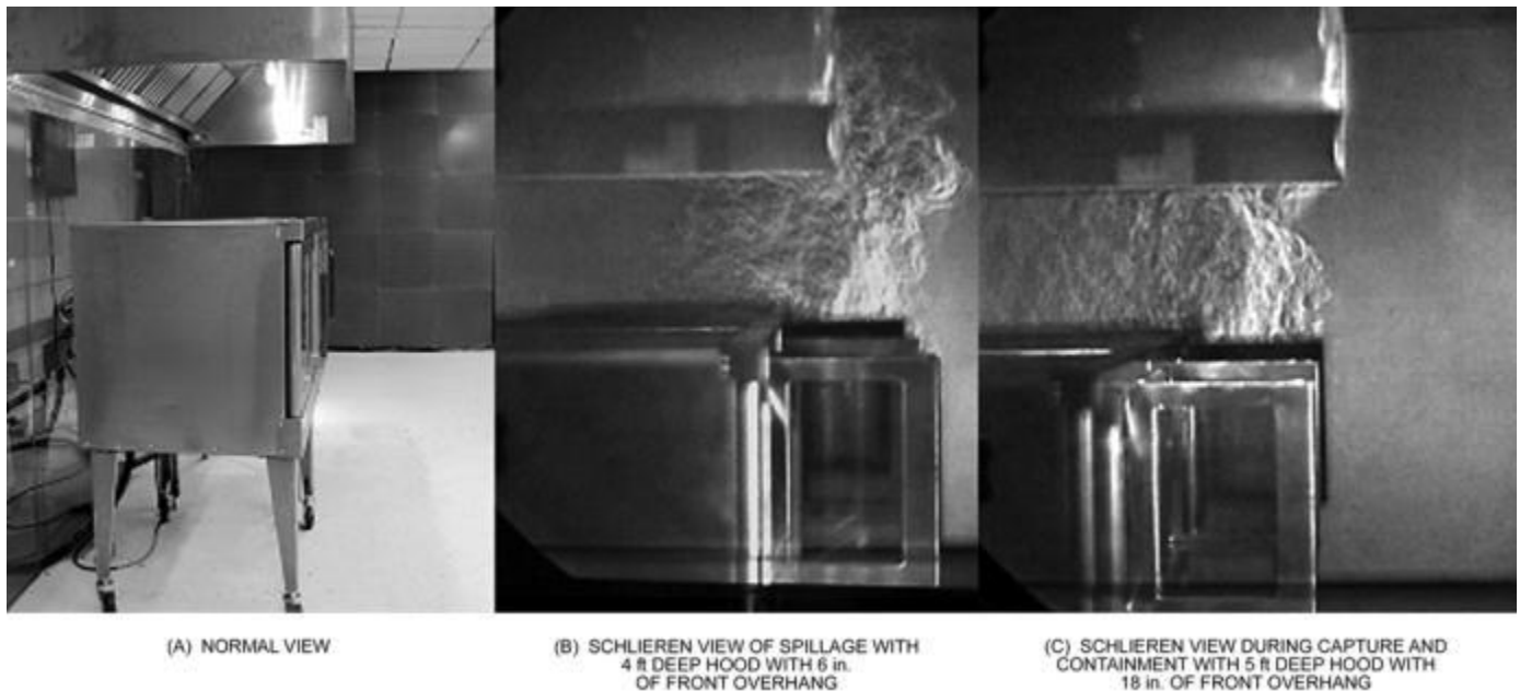
Figure 10. Three Ovens under Wall-Mounted Canopy Hood at Exhaust Rate of 3400 cfm (Swierczyna et al. 2006)
