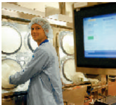
The glovebox is maintained under negative pressure.
