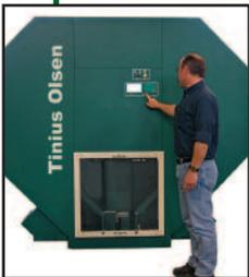
Our model IT406 and model IT542 Impact Testers, with available energy capacities of 406J and 542J respectively, feature heavy-duty construction and an interchangeable striker to easily change between Charpy, Izod, and tensile impact testing. The proper accessories allow these machines to operate in accordance with ASTM E23 and other similar international standards, along with a fully enclosed and interlocked model to meet the requirements of CE directives. These machines also feature a
