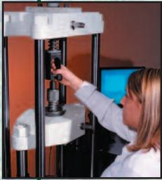
Tinius Olsen's line of versatile hydraulic testing machines can perform a diversity of materials test routines that meet ASTM, ISO and other international testing specifications, including tensile, compressive, flexural, and shear tests. These machines are available at seven standard load tier points, namely, 150 kN (30,000 lbf), 300 kN (60,000 lbf), 600 kN (120,000 lbf), 1,000 kN (200,000 lbf), 1,500 kN (300,000 lbf), 2,000 kN (400,000 lbf), and 3,000 kN (600,000 lbf).
