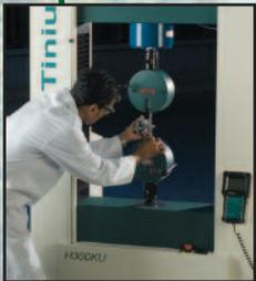
For those applications that require a larger testing area, faster test speed, or longer test stroke than can be achieved on a hydraulic testing machine, Tinius Olsen also has a range of high force electromechanical testers, with capacities of 100 kN (22,000 lbf), 150 kN (30,000 lbf), 200 kN (45,000 lbf), and 300 kN (60,000 lbf). These can also use the same accessories and software to complete the test system.
