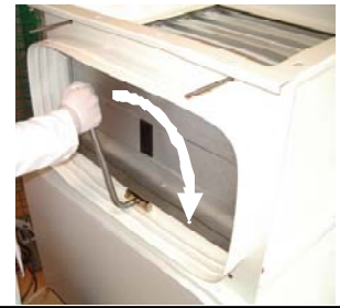
Clamping by cam with gasket compensator
