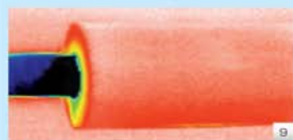
Fig. 9 Infrared photo shows thermal energy emitted from PU foam (45 kg/m 3 ) insulated on low temperature pipe before water absorption test, which shows a very good insulation performance of dry PU foam insulation.
