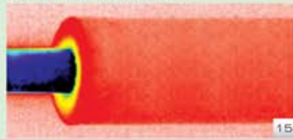
Fig. 15 Infrared photo shows thermal energy emitted from Aeroflex insulated on low temperature pipe after 20 minutes of water absorption test, (ASTM D 1056 water absorption approx. 4% by weight) which shows good thermal insulation performance.
