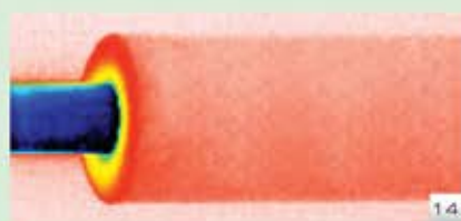
Fig. 14 Infrared photo shows thermal energy emitted from Aeroflex insulated on low temperature pipe before water absorption test, which shows very good thermal insulation performance of dry Aeroflex insulation.
