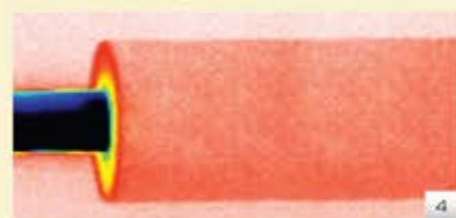
Fig. 4 Infrared photo shows thermal energy emitted from the fiberglass insulated on low temperature pipe before water absorption test, which shows good thermal insulation performance of dry fiberglass insulation.
