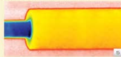
Fig. 5 Infrared photo shows thermal energy emitted from the fiberglass insulated on low temperature pipe after 20 minutes of water absorption test, (ASTM D 1056 water absorption approx. 400% by weight) which shows poor thermal insulation performance of wet fiberglass insulation.
