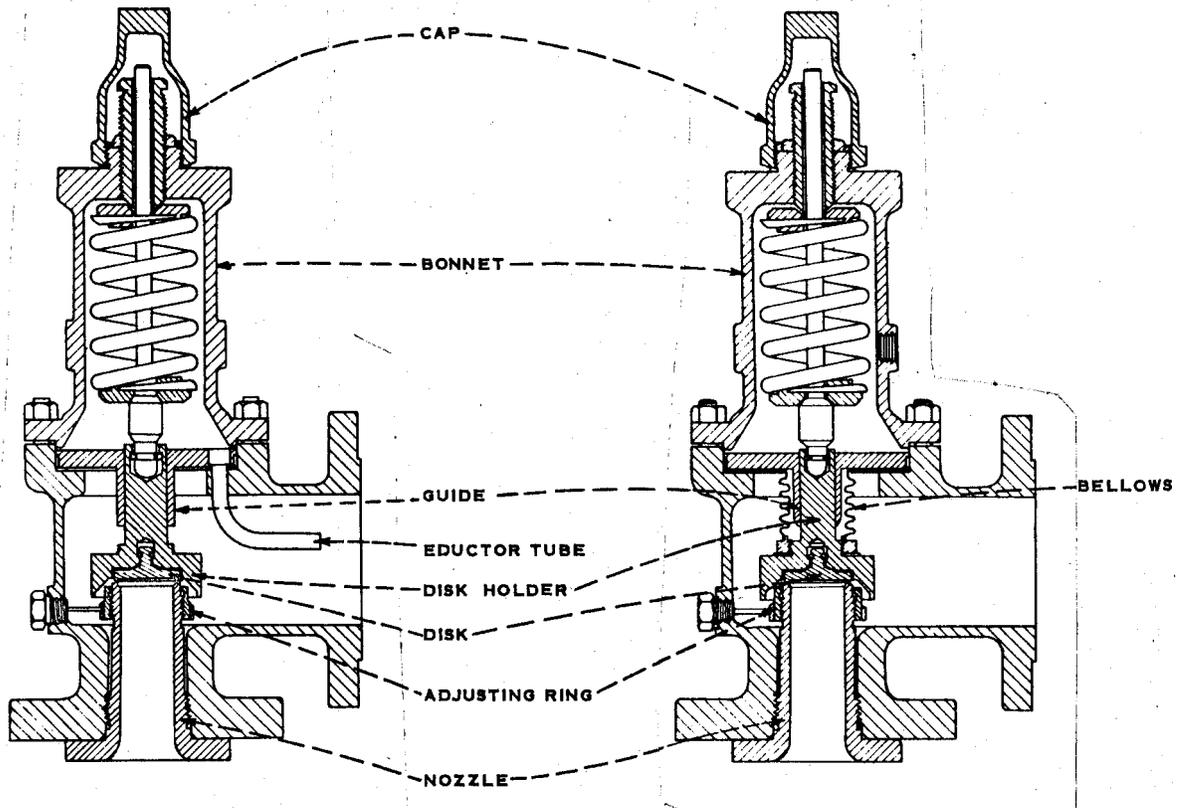
FIGURE 1 - TWO TYPES OF RELIEF VALVES
