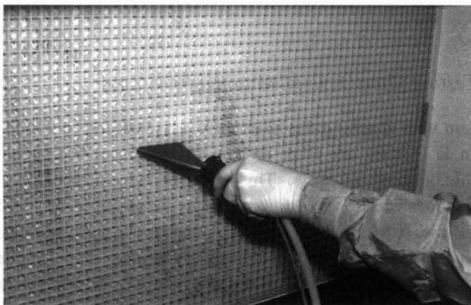
Figure 12.7 Scanning a filter
