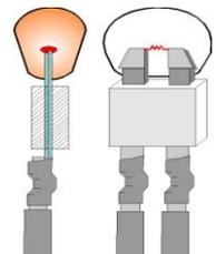
**FirePro®**: the electrical activator is made of a simple and reliable heat element enclosed inside a steel metal housing, which contains the aerosol compound in solid form.
