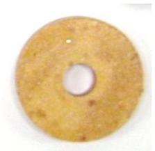
The chemical composition, is non pyrotechnic, as indicated in the MSDS, and is classified as Class 9.1 (Miscellaneous, solid, n.o.s. no otherwise specified), aviation regulated solid material. It does not contain nitrocellulose or nitroguanidine or any derivate of cellulose, thus it is not subject to the disadvantages related to pyrotechnic materials; its life time (certified by accredited laboratories such as Kiwa ) is minimum 15 years.
