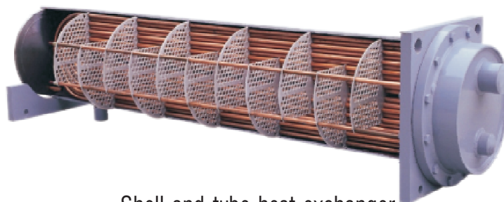
Shell and tube heat exchanger
