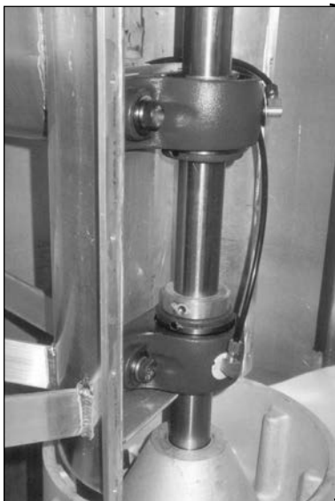
All clamshell fans feature removable bearing covers.
