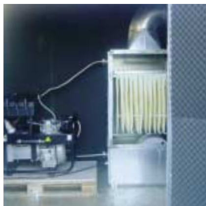
Camfil Farr's proprietary rig for generating diesel fumes during the testing of air filters in accordance with Revised EN 779:2002.
