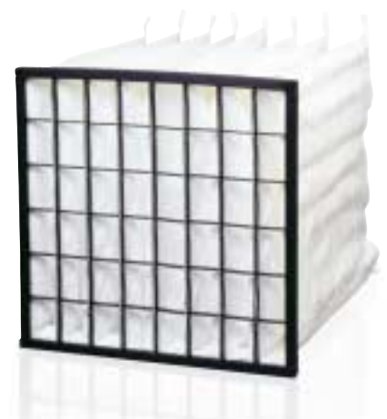
Camfil Farr's Cam-Flo, a P-labelled synthetic filter with fine fibres whose performance stays constant. This is the first well-functioning synthetic filter on the market. After discharging, it will have an efficiency of 50% and the filter will still be correctly classed as F7.
