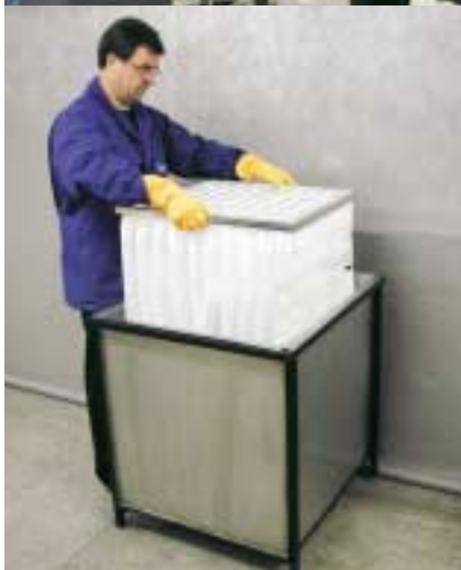
The VTT testing institute in Finland. Discharging an electrostatic filter with isopropanol.
