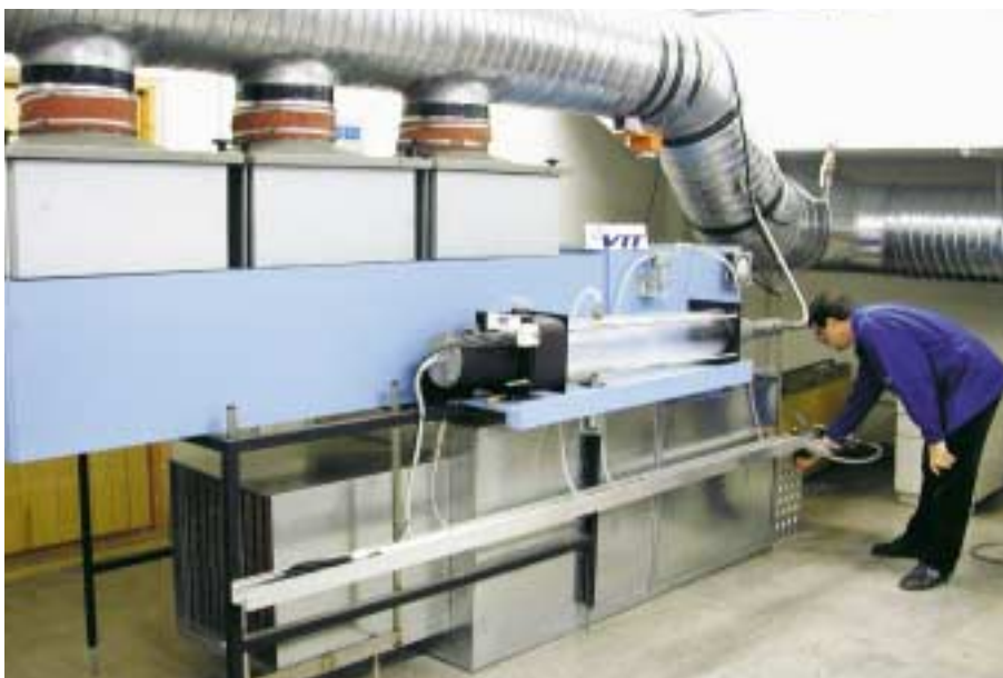
Test rig at VTT in Finland for testing filters in accordance with REVISED EN 779:2002.
