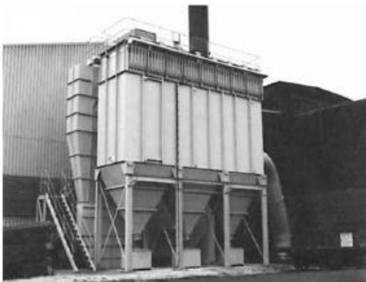
Figure 6.25 Fabric filter with vertical elements
