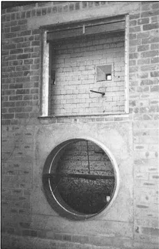
FIG. 4a FIRE DAMPERS BEFORE THE FIRE RESISTANCE TEST
