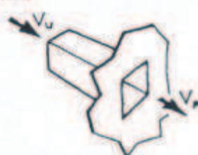
FITTING No. 501 RECTANGULAR OR CIRCULAR ABRUPT ENTRY
