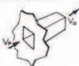
FITTING No. 511 RECTANGULAR OR CIRCULAR ABRUPT EXIT
