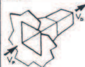
FITTING No. 512 RECTANGULAR FLARED EXIT
