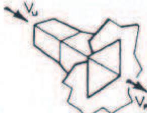
FITTING No. 502 RECTANGULAR FLARED ENTRY
