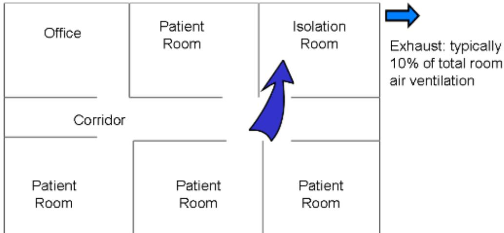
Specific areas should be under negative pressure to prevent cross contamination to other areas of the building (0.001" W.G. or 100 FPM inward velocity)
