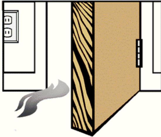
With door ajar, approximately  $\frac{1}{4}$ " to  $\frac{1}{2}$ " place smoke generator near opening, flow through opening should be uniform and constant
