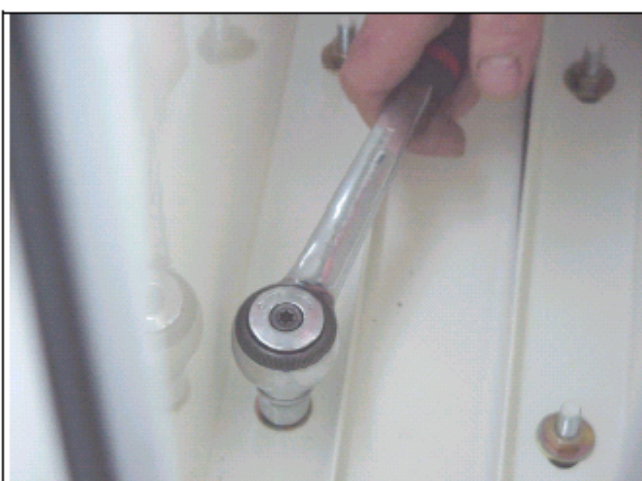
Tightening through a clutch key is possible, do not tight yet
