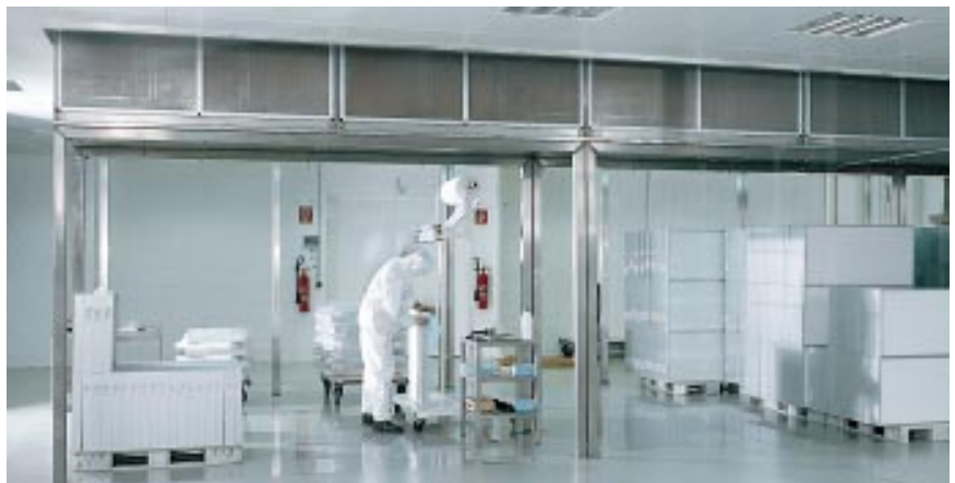
Final inspection and packing area in one of our plants. This area is classified in accordance with ISO 5, (M 3.5 Fed. 209E) to meet the requirements of our most demanding customers.
