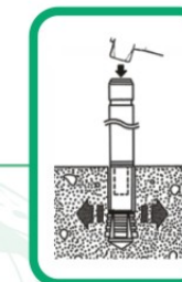
Using setting tool to drive Anchor body until flushed with concrete surface
