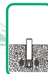
Anchor is set and ready to weld with various metals
