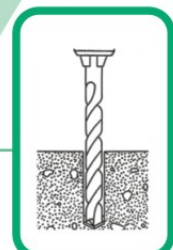
Drilling hole with recommended diameter and depth
