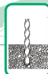
Drilling hole with recommended diameter and depth
