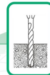
Drilling hole with recommended diameter and depth
