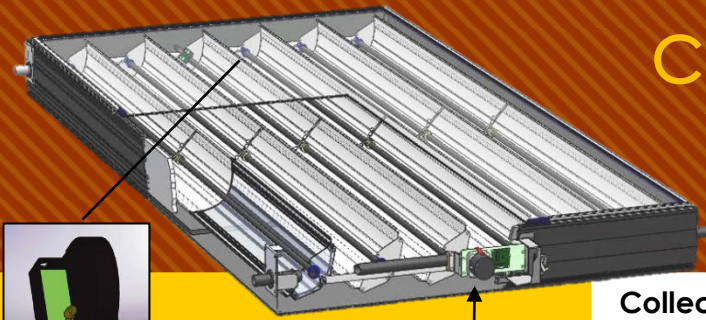
SMARTRAC™ Photo Sensor (tracks the sun)
