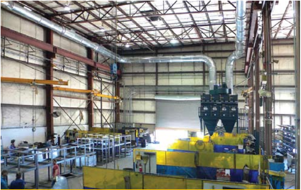
GS48 on weld fumes with integral HEPA
