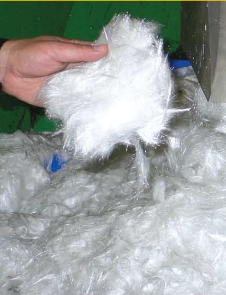
The fiberglass pictured is used in manufacturing the hulls of these boats.
