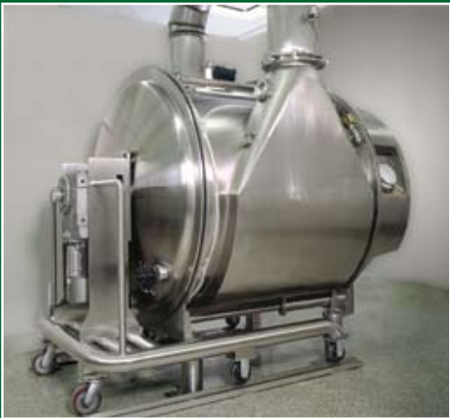
Farr BIBO dust collectors pulls dust off of tablet coaters like this Spectrum Coater from Thomas Engineering.
